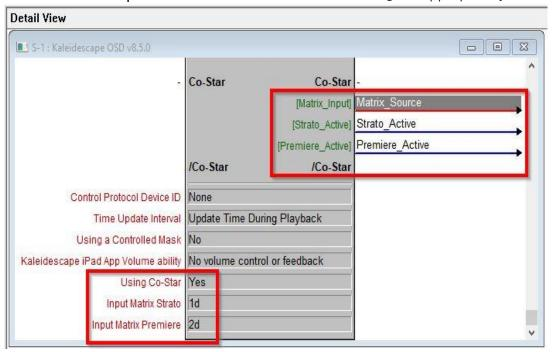
2. Set the active input on the NVX encoder by connecting the **Matrix\_Input** output signal to the **VideoSource** input signal of the NVX encoder.
